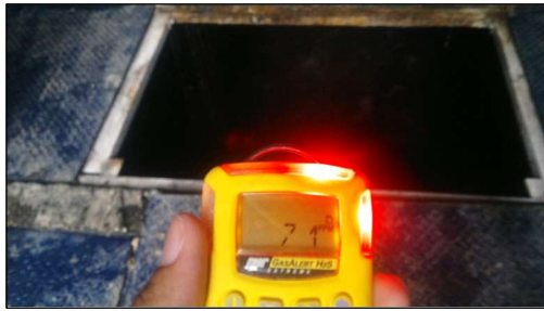
Figure 7. Hand held gas monitor detecting very high H 2 S concentration above opening of wet well enclosure
