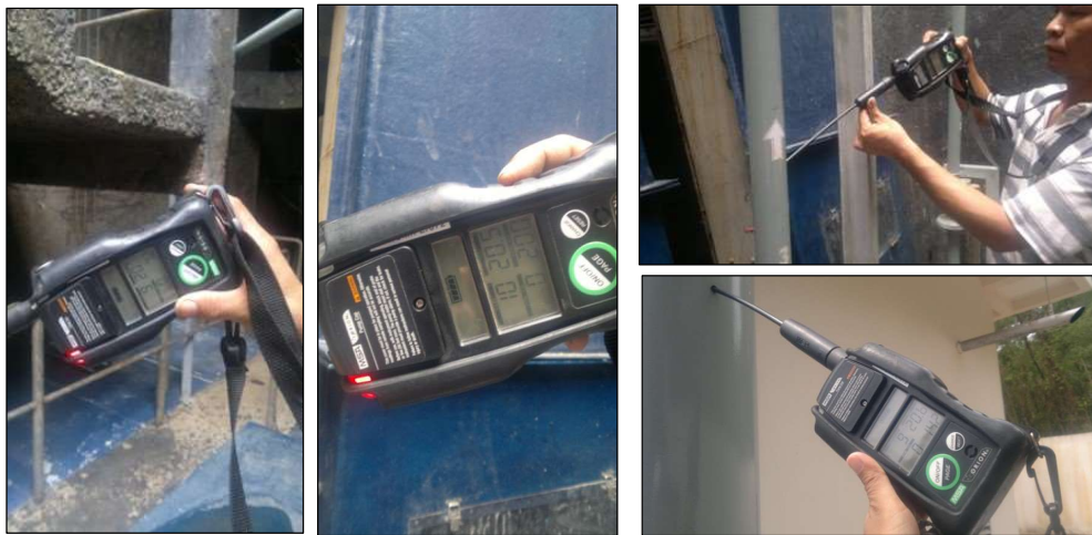
Figure 10. H 2 S levels measured in the incoming sewage at the channels, mechanical screens/skips and the inlet raw odorous gas to be abnormally high in some measurements recorded 200ppm H 2 S which is the limit of the H 2 S meter used.
